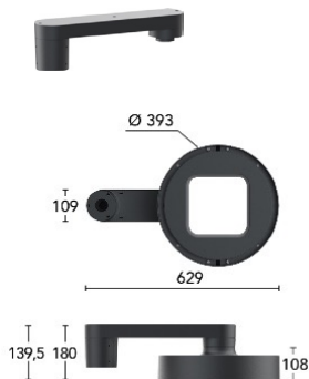
LATERAL pole connection
